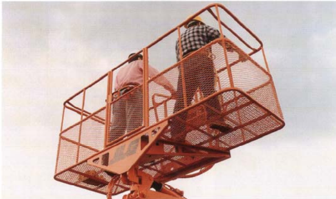
Large 96" (2.44m) wide basket and powered hydraulic rotator are standard equipment for improved worker productivity.
