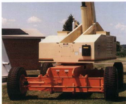
Extendable axles help reduce overall machine GVW over fixed axle designs which increases overall machine mobility and transportability and decreases wear on system components.
