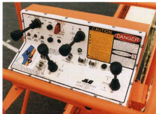
Complete machine operation is provided from the platform control station which includes the load management indicator system.
