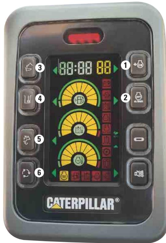
**4 Swing Priority Mode** gives swing flow priority and is especially suited for crowding the sidewall while digging and extreme swing angle loading.
