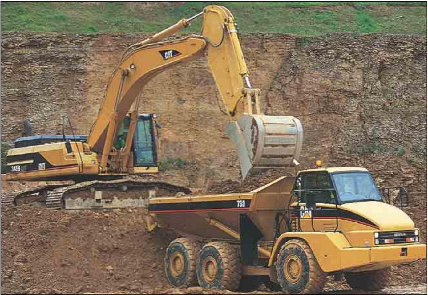
**Optimum pass match design.** Five to six passes under two minutes, matched to the Cat 735, gives you maximum systems production at the lowest cost per ton of material moved.
