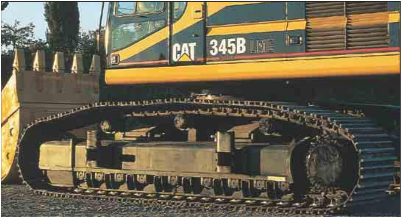
**Variable Gauge (VG)** heavy-duty, H-shaped long undercarriage provides ease of transport and a stable platform when working on a variety of sites. With 600 mm standard track shoes, track roller frames can be retracted for less than three meter transport width. A variety of standard and heavy duty track shoes are available for various underfoot conditions.
