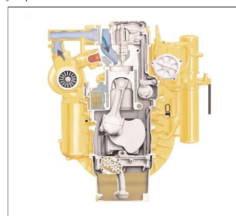
The Cat 3116 Diesel Engine is a six cylinder, four-cycle design that provides long, effective power strokes for high torque and more complete fuel combustion.
