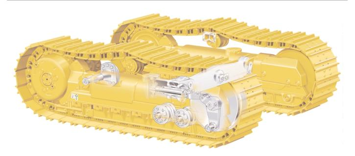
**Oscillating Undercarriage** allows movement of each track independent of main frame.
