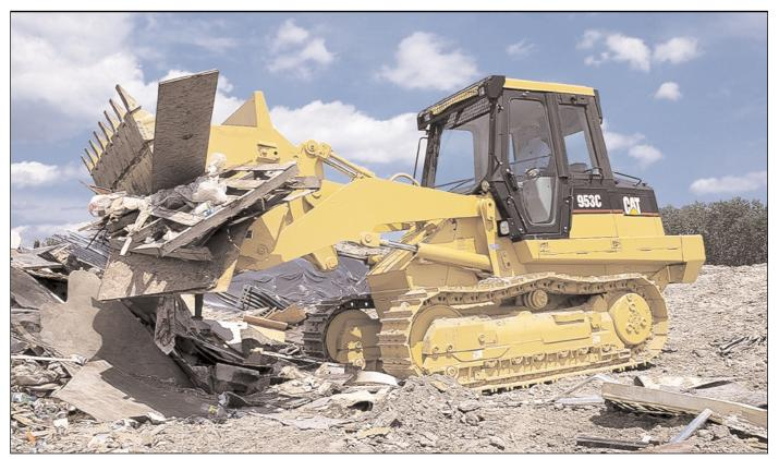
Waste handling attachments provide added versatility and are designed to make the 953C perform well in sanitary landfills, transfer stations and other waste handling applications where the machine spreads, compacts, sorts, shreds and crushes materials.
