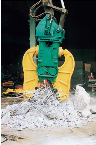
Photo showing is JCYC19R with short cutters and smashing points.
