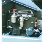
Excellent Access to Filters Stable Travel by Absorbing Vibration facilitates Servicing when Passing over Rough Terrain or Steps
