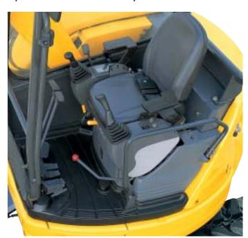
Reclining suspension seat and seatbelt Easy-to-clean, durability and ability to recline keeps operator comfortable.
