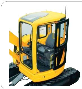
Upper-rail type sliding door opens and closes smoothly even in tight working conditions.
