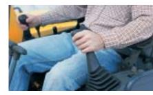
The control lever uses a fine-response PPC, to translate even the most subtle hand signals into motion. Short lever throw ensures comfortable operation.
