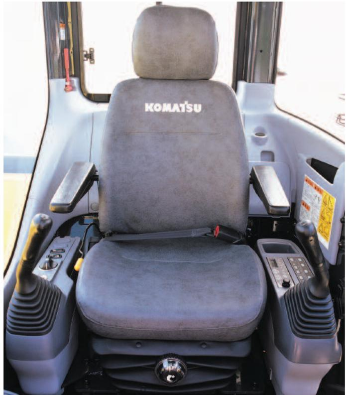
**Suspension seat with retractable seat belt**
