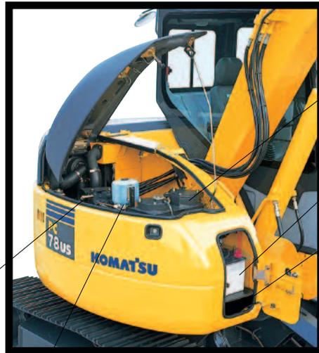
Smaller and longer lasting hydraulic oil filter Ecowhite element.
