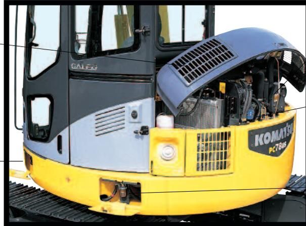
Air cleaner with easily replaceable element.
