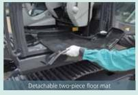
Detachable two-piece floor mat with handles for easy removal. A floor drain is located under floor mat.
