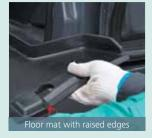
Floor mat's raised edges help keep the cab floor free of mud, simplify cleaning.
