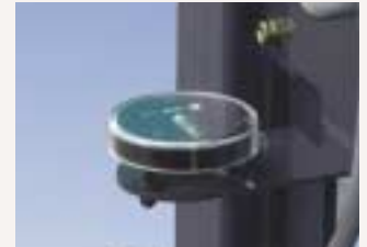
● Level indicator that shows degree of machine tilt
