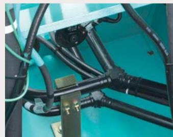
Rigorous inspections for pressure loss are performed on all components of the hydraulic piping, from the first spool of the control valve to the connectors. This regimen, combined with the use of a new high-efficiency pump, cuts energy loss to a minimum.
