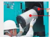
The large-capacity element features a double-filter structure that keeps the engine running clean even in dusty environments.
