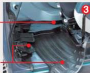
3 Detachable two-piece floor mat with handles for easy removal. A floor drain is located under the mat.
