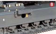
8 Special crawler frame design is easily cleaned of mud.
