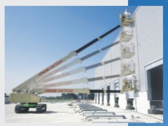
The horizontal/vertical steering and control system affords synchronous horizontal and vertical movements during work with just one joystick.
