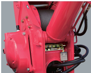
9 Automatic stop for leaving minimum wire rope
