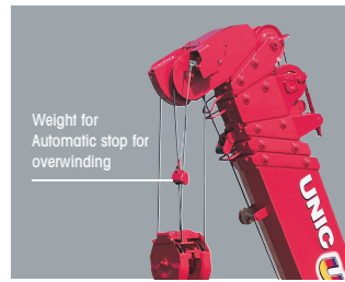
8 Automatic stop for overwinding
