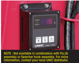
5 Automatic stop for overloading KM-100 W376C, W546C, W547C
