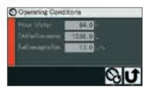
Fuel consumption per operating hour is computed, and the result is displayed on the LCD monitor. This information suggests refuelling timing, and guides energy-saving operation and efficient job management.
